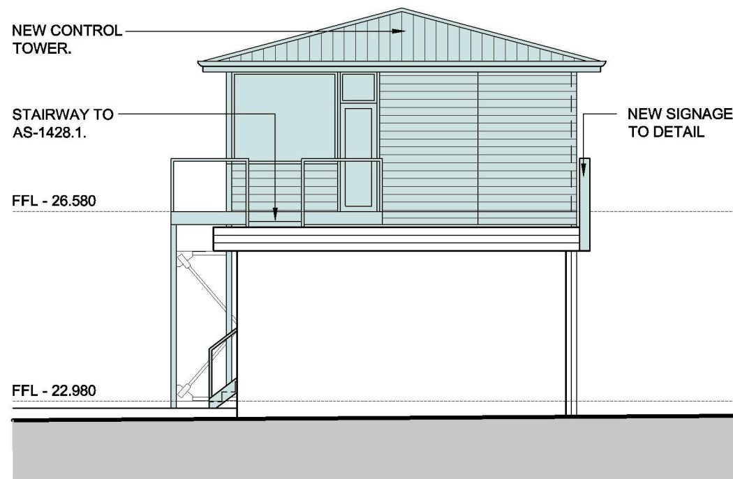
BUILDING B - WEST ELEVATION SCALE 1:100
